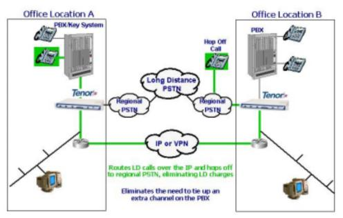
With the Quintum Tenor, companies with multiple locations can easily implement "hop-off" calling that leverages the corporate IP network to bypass long distance carriers – switching calls onto the local PSTN from the location closest their ultimate destination
