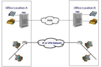
Conventional office-to-office voice communications are provisioned via the public switched telephone network (PSTN) using PBX equipment.
