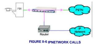
Calls that are received from the IP network can be routed to either the PBX (based on matching an existing LDN) or to the PSTN (based on matching an existing Hop-Off DN).
