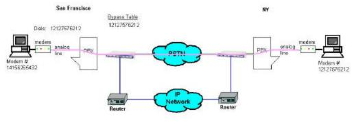
FIGURE II-9 MODEM CALL BYPASS
