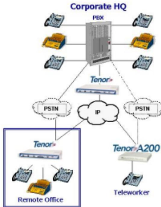
*With Quintum's Tenor solution, remote offices and teleworkers can be easily and inexpensively connected to corporate PBXs for full-function phone services*
