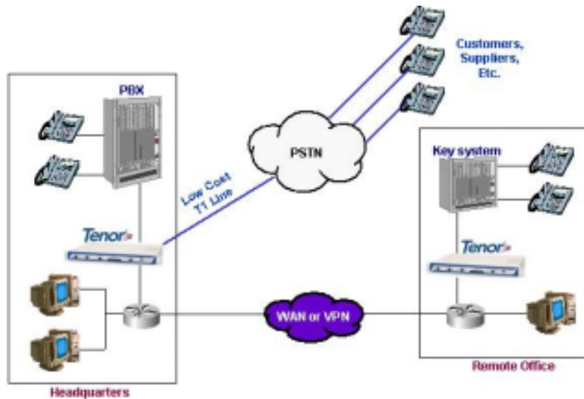
Using Quintum's Tenor switches, outbound calls from smaller offices can be routed over existing WAN or VPN data connections to headquarters first -- where they can then be sent to the PSTN over a T1. This yields substantial savings on telecom costs. It also allows calls between locations to be transported free of charge.
