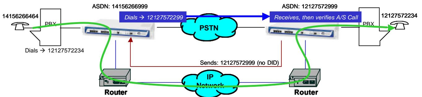
FIGURE II-2: SELECTNET/TASQ SAFETY NET (ANALOG-TO-ANALOG TENORS)
