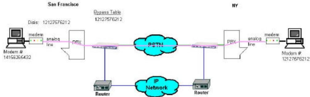
**FIGURE II-9 MODEM CALL BYPASS**
